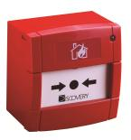
A seven-segment DIL switch enables addressing of each call point at commissioning stage. When operated, the manual call point interrupts the polling cycle for a fast response. Bi-coloured LEDs indicate isolate and normal conditions.
