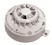
The XP95 Intrinsically Safe (IS) Heat Detector operates by measuring heat levels with a single thermistor which gives an analogue value output proportional to the external air temperature.
