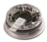
The Discovery Sounder Visual Indicator Base makes full use of the Discovery protocol. For ease of commissioning a 'Magnetic Wand' can be used to test and adjust each sounder locally.
