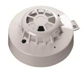
The Discovery / Soteria UL Heat detector monitors temperature by using a single thermistor which provides a voltage output proportional to the external air temperature. Ideal for environments that are dirty or smoky under normal circumstances. Well suited to warehouses, loading docks and parking garages.
