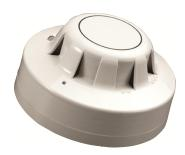
The Series 65 Optical Smoke Detector uses light sensing technology to "see" smoke entering the chamber. The external detector moulding is identical to that of the ionisation detector and has an indicator LED which is clear in quiescent state and produces a red light in alarm.
