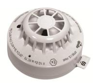
The XP95 I.S. Heat Detector operates by measuring heat levels with a single thermistor which gives a count output proportional to the external air temperature.
