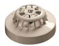
The Series 65 Heat Detector monitors temperature by using a dual thermistor network which provides a voltage output proportional to the external air temperature.
