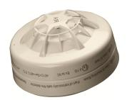
The Orbis I.S. Heat Detector monitors temperature by using a single thermistor provides a voltage output proportional the external to temperature.
