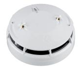
The Soteria UL Multi-Criteria Detector (Smoke/Heat) uses Purelight® and is fitted with two thermistors for detecting heat. It can be switched to detect smoke, heat or a combination of both; offering greater flexibility, fast detection and advanced false alarm management. This detector is a direct replacement for the 58000-750 Discovery UL Multi-sensor Detector
